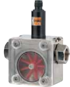
Paddle Wheel - Pulse/Analog Output Delrin, PVDF, brass, stainless steel Model: DRH-...F, DRH-...L
